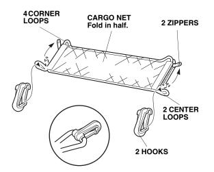
6. Attach the hooks to the two anchors in the floor, and attach the corner loops to the hooks on the rear side lining.
